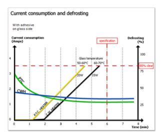
Some data related to current consumption in relation with defrosting and maximum glass temperature measured on the technologies we produce today.
